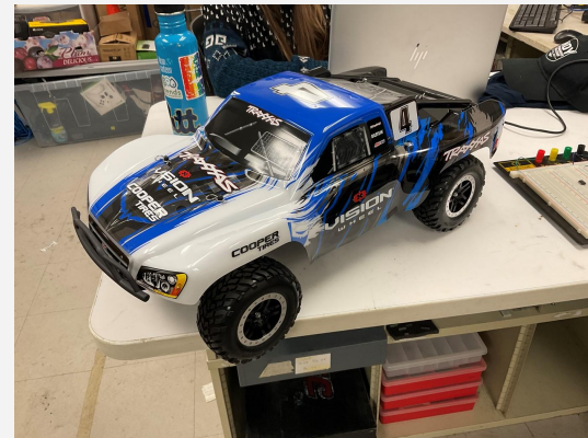
FTTenth base chassis - will strip it and make autonomous
